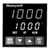
SET - LED indicates - that the controller is in configuration mode. When flashing, controller is in manual mode AT - LED indicates that the controller is in selftune mode. When flashing, controller is in pretune mode ALM - LED informs that alarm is on. "1" - displays output 1 status.
